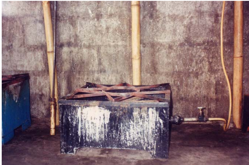
Photo 4.6: Commercial biogas stove used for preparing sweetmeats
