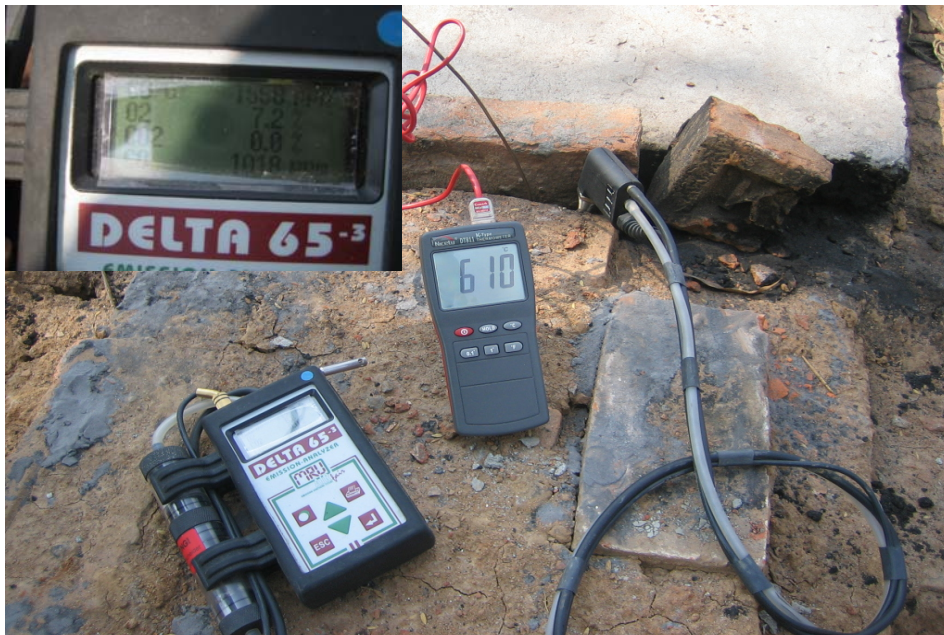
Fig. 13 A view of the measurement of CO, O 2 and temperature in flue gas (a MRU AirFair Emission Monitoring Device)
