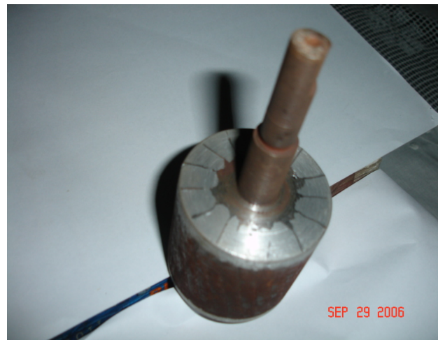
Fig. 7 Rotor fabricated with iron insertion
