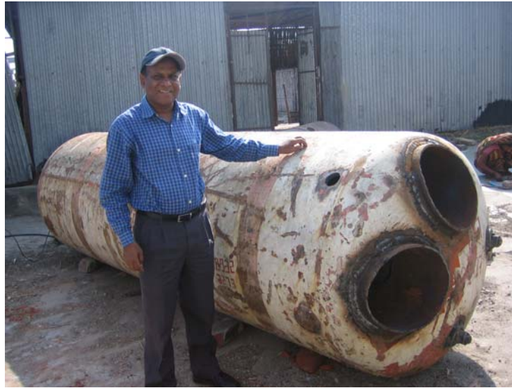
Photo 6. Local made Lancashire type steam generator
