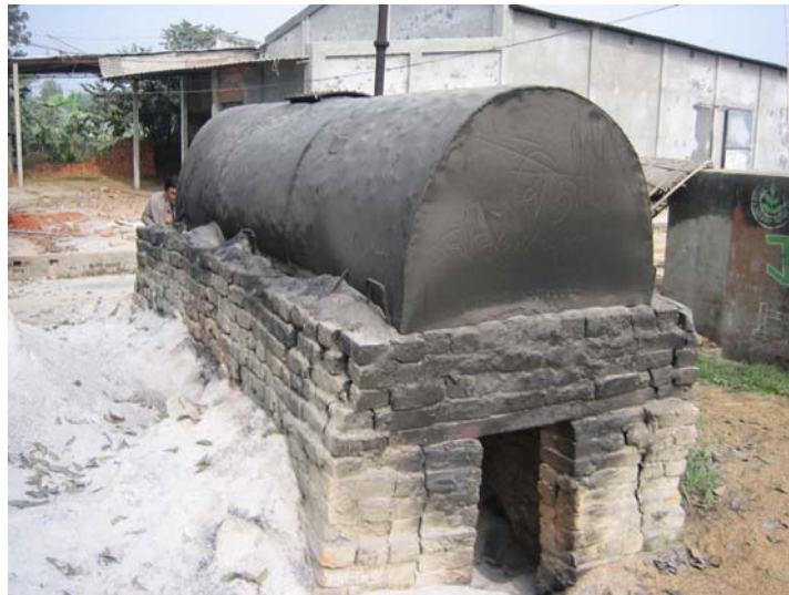
Photo 4. Local made semi-cylindrical steam generator
