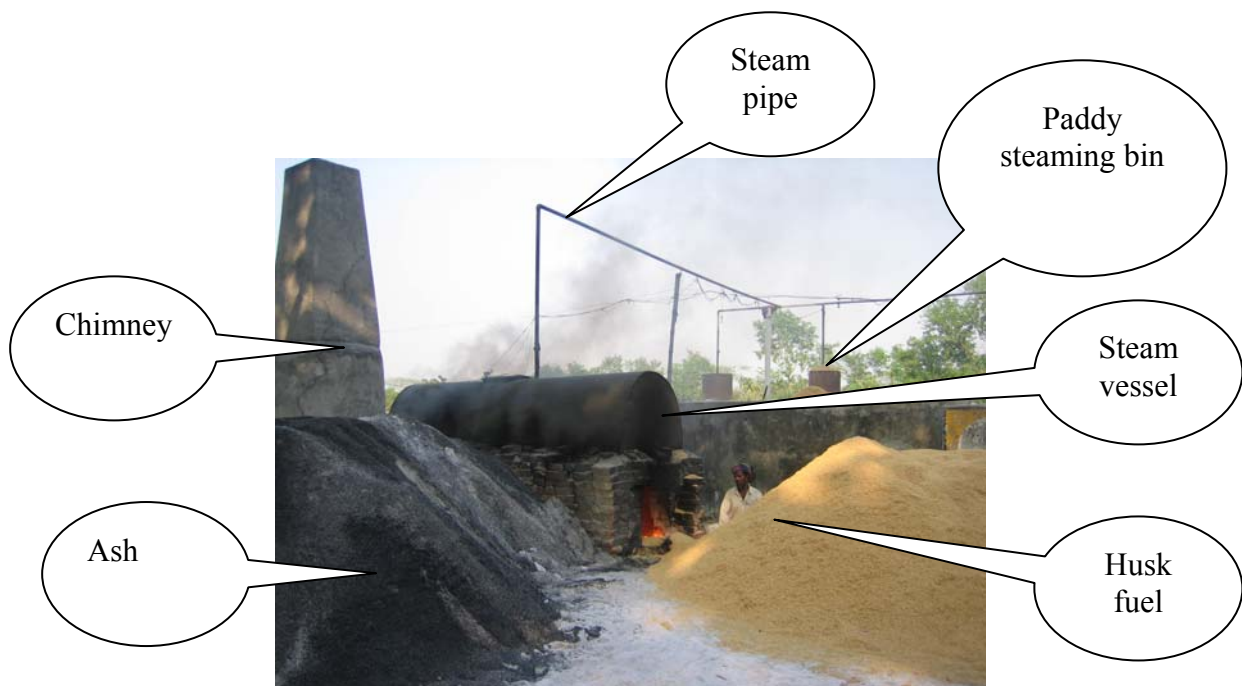
Photo 2. A conventional rice parboiling system
