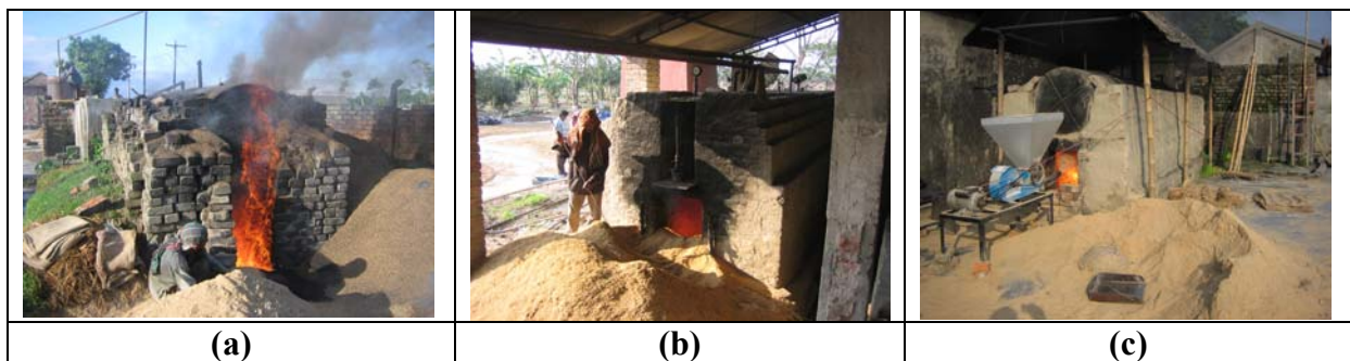
Photo 13. Showing different types of fuel feeding systems (a) Hand feeding (b) Spoon feeding (c) Blower feeding
