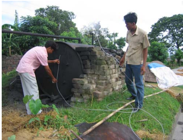
Photo 1. Measuring the water level by using siphon tube
