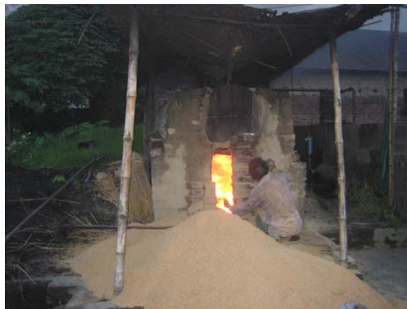
Photo 15. Showing large opening for fuel feeding causes high excess air-fuel ratio
