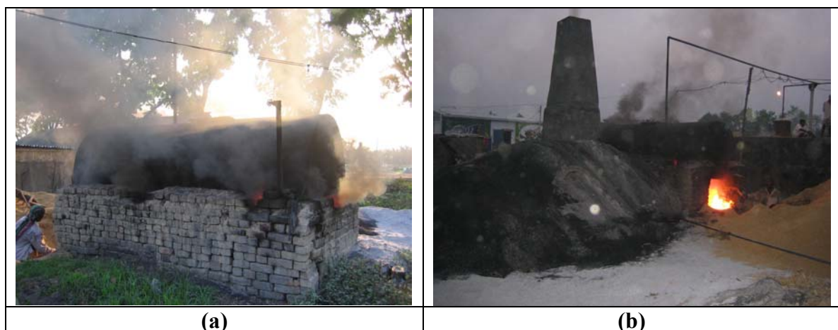
Photo 12. Showing the practices of chimney use in different rice parboiling systems (a) no chimney installed (b) inadequate chimney height and improper installation of chimney to the furnace
