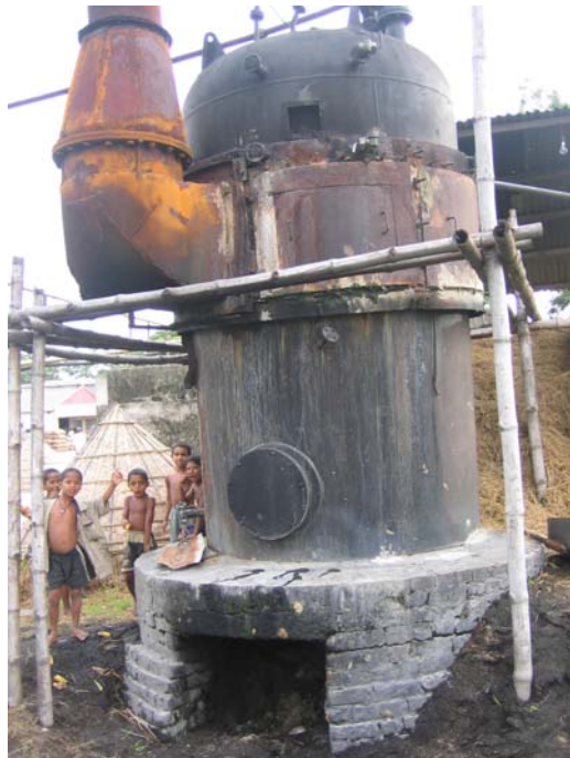
Photo 9. Vertical tubular boiler collected from ship
