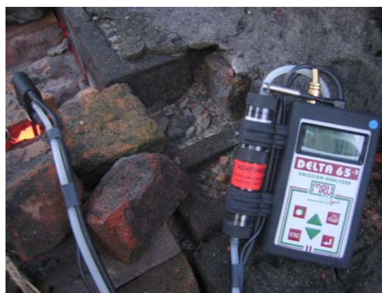
Photo 16. Showing measuring carbon monoxide and oxygen content of the flue gas by a digital flue gas analyzer
