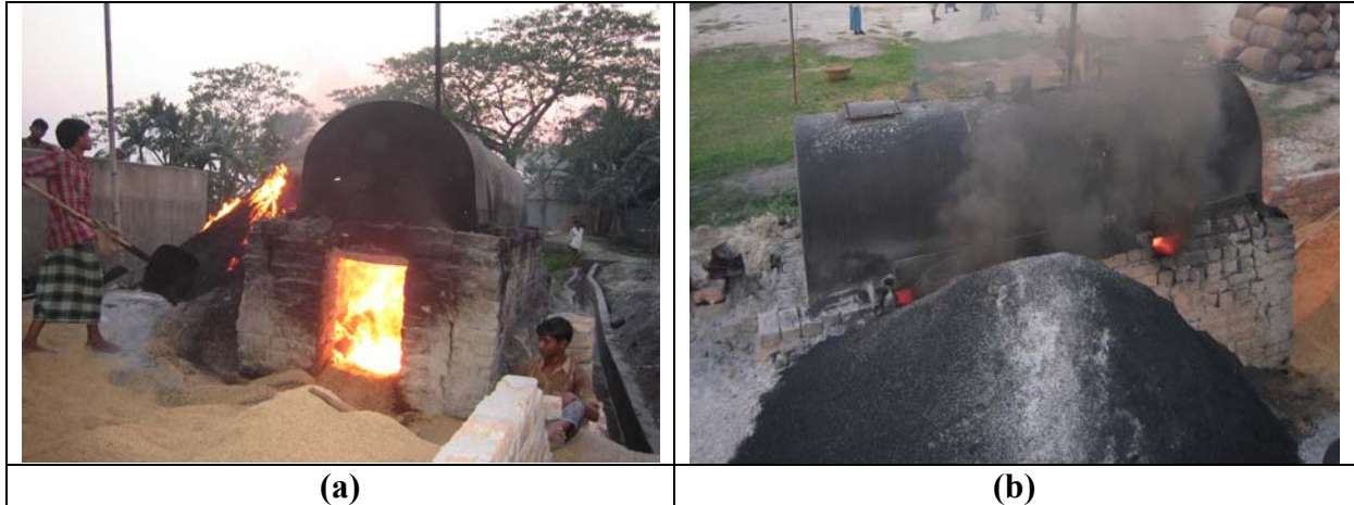
Photo 14. Heat loss through ash disposal (a) ash disposal during burning of husk (b) incomplete burnt ash disposal
