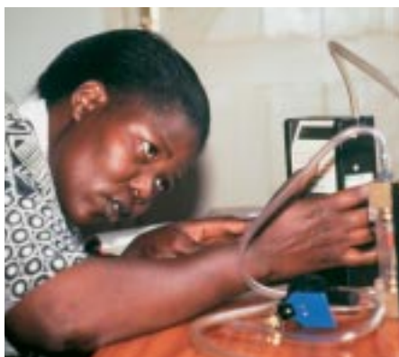
Measurement of particles requires great care at all stages. Shown here are pump calibration prior to testing in a rural Kenyan home, and removal of an exposed filter from a desiccator prior to weighing on a microbalance.
