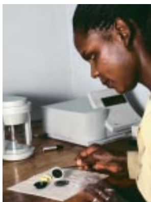
Measurement of particles requires great care at all stages. Shown here are pump calibration prior to testing in a rural Kenyan home, and removal of an exposed filter from a desiccator prior to weighing on a microbalance.
